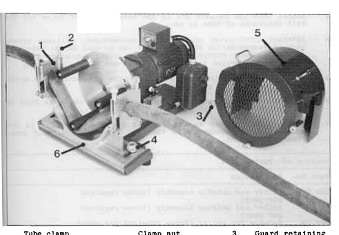
The LHRS and LHRV will only start with the guard in position, when a projection operates the interlock. When fitted, set the forward/off/reverse switch to produce flow in the required direction, then press the green button to start.
