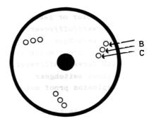
To change the position of the rollers, remove the nut at the back of the rotor, withdraw the complete roller assembly, locate it into the appropriate hole and then replace and tighten the retaining nut.
