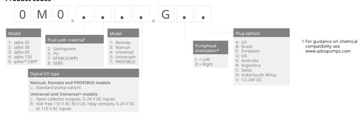
\* The pumphead side location is required when ordering. The left/right perspective assumes the user is looking at the front of the pump. The pump in the dimensions diagram is considered a pumphead located to the left.
