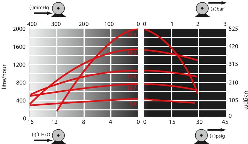
For critical applications determine flow under operating conditions. Flow can vary due to tube tolerances and system configuration
