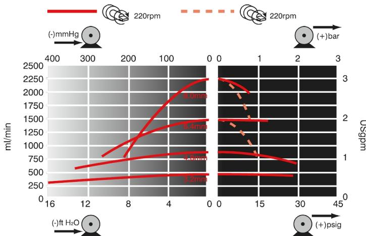
Maximum duty pressure with 6.4mm and 8.0mm bore tube is 1bar. Maximum duty pressure with other tube bore sizes is 2bar.
