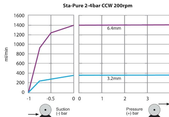
To achieve 4 bar pressure the pump must rotate counter-clockwise
