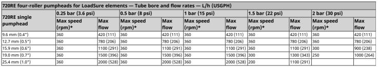
\*The maximum speed is reduced at increased discharge pressures to ensure safe running of the pump
