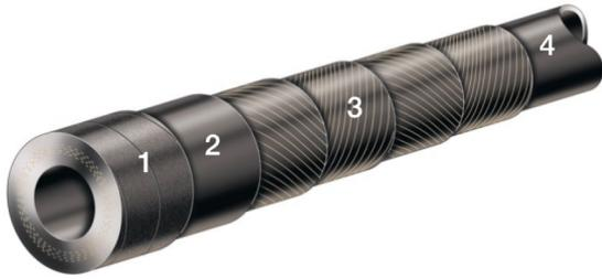
1. Rough hose surface prior to machining.
