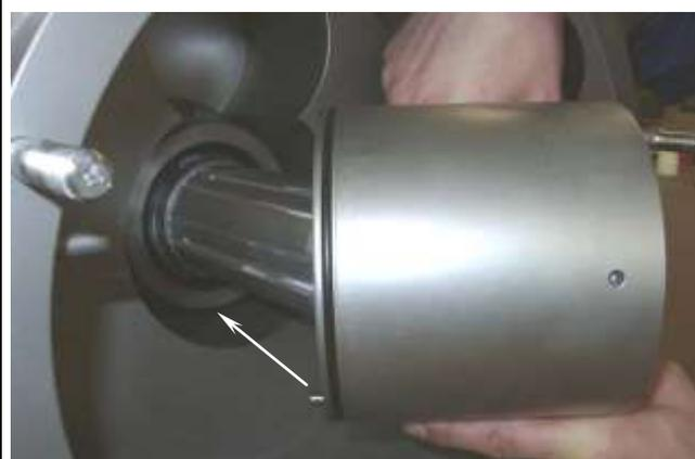
The pin has to be fixed in the groove in the pump housing
