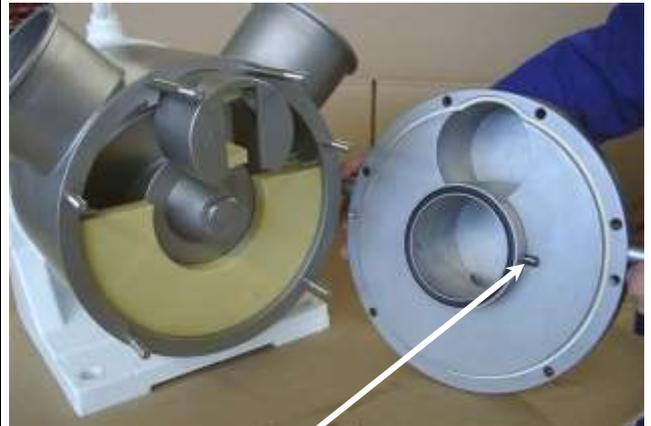
The pin of the front bearing has to be fixed of the groove in the front cover
