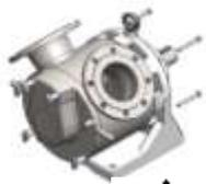
Remove the screws on the bearing block. Turn the housing by an angle of 45° to the left or right. Tighten the screws again. (45 Nm)
