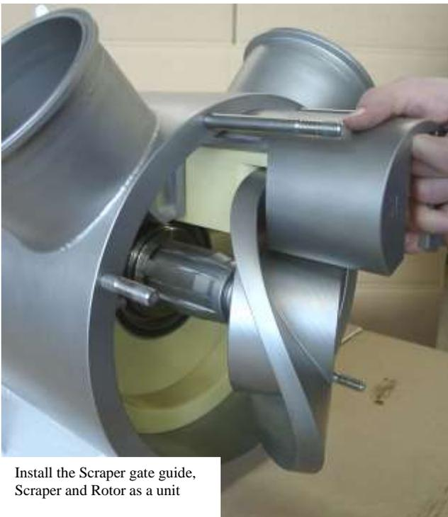
Install the Scraper gate guide, Scraper and Rotor as a unit
