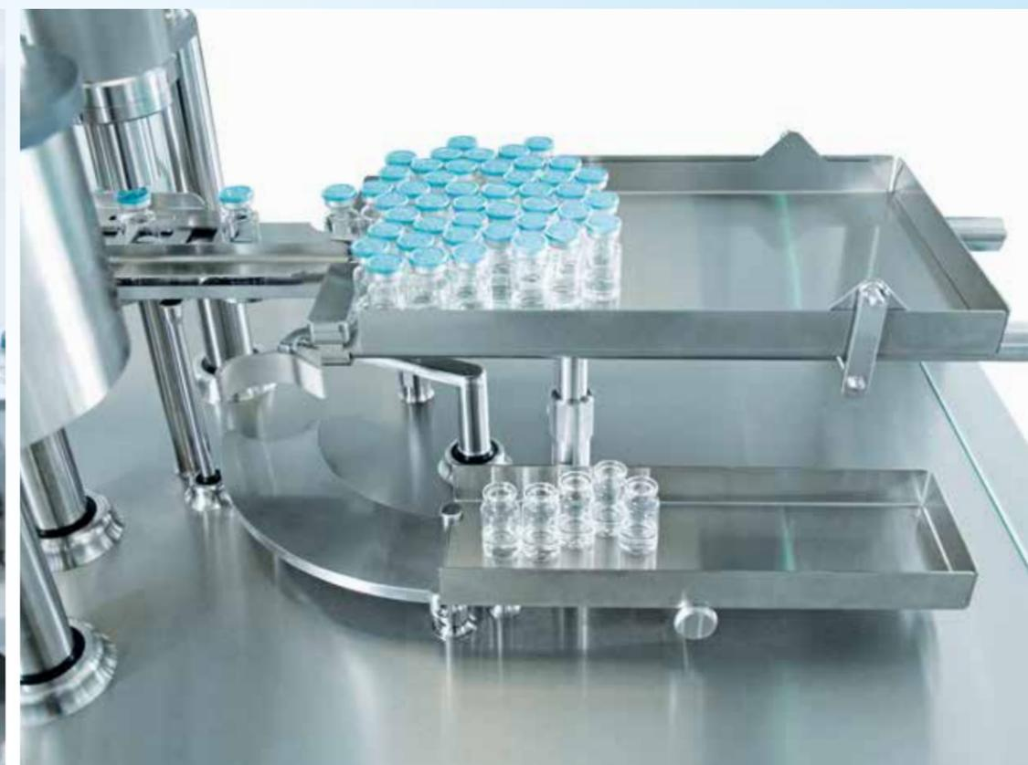
When supplied with in-line check weighing, the FPC60 offers unique dynamic prime, no intervention initial calibration and dynamic recalibration, meaning no waste in the batch start up process and confirmation every vial, from first to last, is filled within specification.
