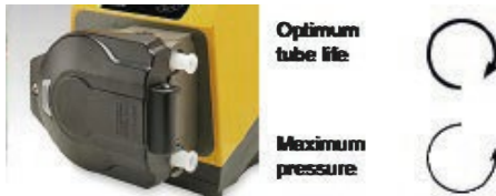
Figure 3 - Rotor direction
