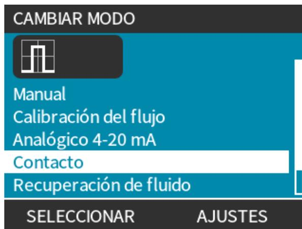
Configurar Contact mode (Modo de contactor)
