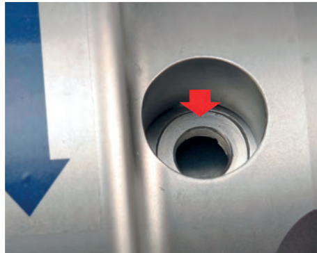
The tapped pump seal housing
