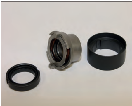
The static face with its O-ring, left, the mechanical seal with one of its O-rings visible and the back bushing
