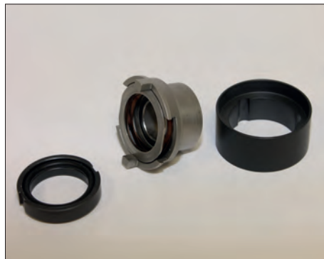
The static face with its O-ring, left, and the mechanical seal with one of its O-rings visible. The surfaces of the two components seen here must come together on reassembly. The back bushing is seen, right
