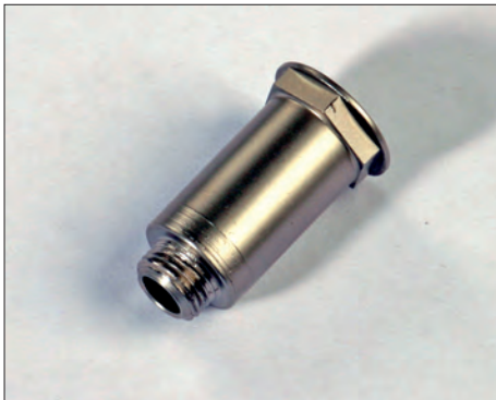
The bent outlet connection piece
