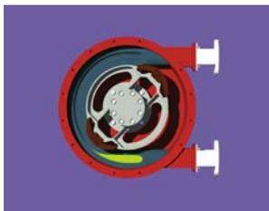
In phase 3, the second pressing shoe will subsequently compress the pump hose. Due to the continuous rotating movement of the rotor not only new product is sucked in, but also the already present product is pressed out by the pressing shoe. When the first pressing shoe runs from the pump hose, the second pressing shoe has already closed the pump hose and the product is prevented from flowing back. This method of liquid displacement is also known as the “positive displacement principle”.
