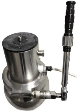
Unlike elastomer diaphragm materials, the following steps are necessary to finish preparing a new PTFE diaphragm:
