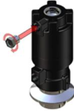
13. Thread the shoulder screw into the assembly. Press shaft towards the pneumatic housing to ensure the shaft flats remain aligned.
