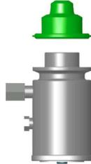
3. Insert the actuator/diaphragm assembly into the valve body.
