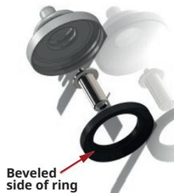
3. Insert the actuator and diaphragm assembly into the valve body.
