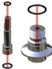
2. Thread the upper housing onto the sleeve.
