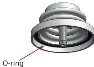
2. Verify that the diaphragm insert is screwed into the diaphragm, just finger-tight.
