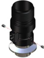
4. Install the inner O-ring into O-ring groove.
