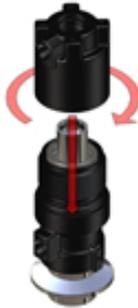
12. Thread the breather vent into the lower housing.
