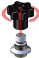
4. Install the O-ring into the groove on the handle.
