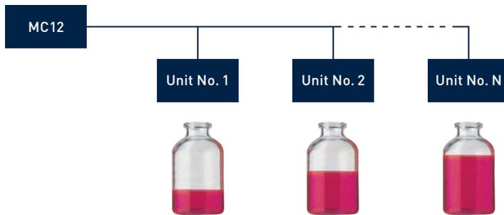
In serial mode, the total fill is made up from the accumulated volumes delivered by each filling station. The fillers can operate with individual tube diameters, thus giving different fill volumes from each filling needle.
