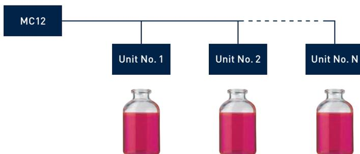
In parallel mode, all connected fillers are synchronized with the same set of parameters. The calibration is carried out individually.
