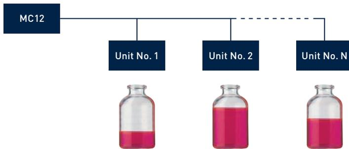
MC12 can control up to 16 fillers regardless of the type. MC12 controls each filler using individual parameters such as fill volume, tube
