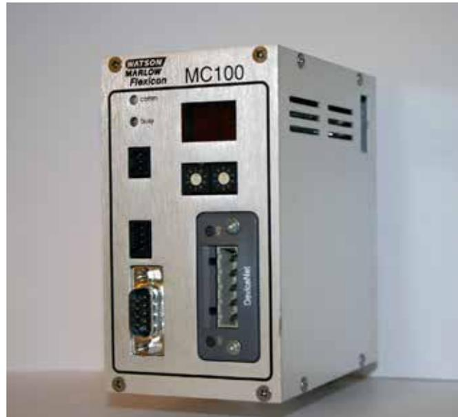
MC100 is a pump control module capable of controlling up to 16 Watson-Marlow Flexicon Pumps. The basic function is to receive filling data (recipes) from a filling line control system through an industrial fieldbus, and to calculate operating values for the pumps and receive/transmit those through a FlexNet protocol.
