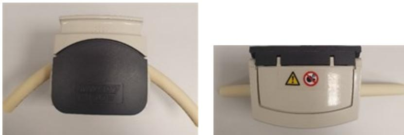
10. If using Marprene or Bioprene, retention the tubing after the first 30 minutes of operation, as the tube may grow in length during this bedding in time. Repeat all previous steps in this procedure to re-tension the tube.
