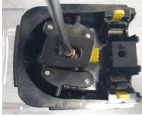
8. Close the pumphead cover and lock by turning the cover fastener  $\frac{1}{4}$  turn clockwise
