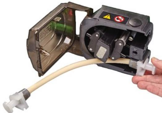
5. Disengage the rotor clutch by fully depressing the yellow clutch button on the side of the rotor hub and turning the hub a few degrees while the clutch button is still depressed. The rotor can now rotate independently of the gearbox and motor for one full revolution. If the clutch re-engages before tube fitting is complete, depress the clutch button again and turn the rotor a few degrees.
