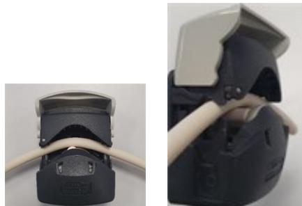
8. Lower flip top to fully closed position, this will automatically tension the tube correctly.
