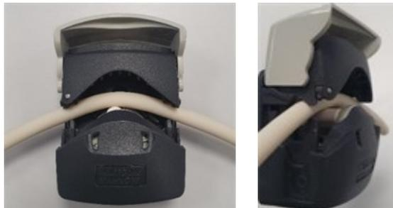
6. Lower flip top cover to fully closed position, this will automatically tension the tube correctly.
