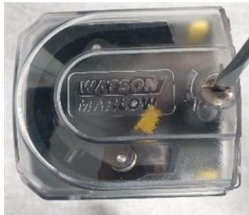
6. Open the cover to its full extent to create maximum clearance for the tube ports.
