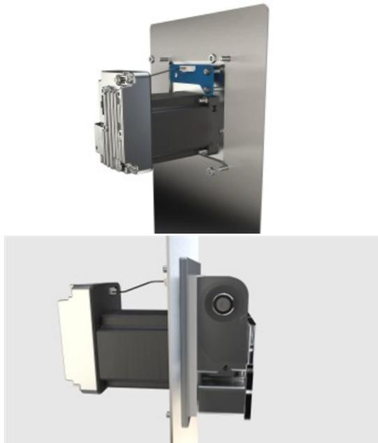
5. Torque the 4 mounting bolts using an alternating pattern to 4.6 Nm.
