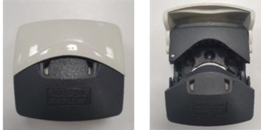
3. Ensure the tube clamps are correctly set for size of tube.
