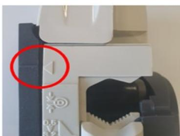
4. Rotate adjusting wheel on the clamp assembly so that the required tube wall thickness aligns with the required tube bore size. Adjusting wheel operates clockwise to lower and anti-clockwise to raise.
