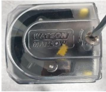
3. Open the cover to its full extent to create maximum clearance for the tube ports.
