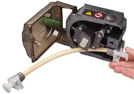
7. Disengage the rotor clutch by fully depressing the yellow clutch button on the side of the rotor hub and turning the hub a few degrees while the clutch button is still depressed. The rotor can now rotate independently of the gearbox and motor for one full revolution. If the clutch re-engages before tube fitting is complete, depress the clutch button again and turn the rotor a few degrees.
