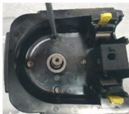
7. Attach rotor hub by lifting dust cover and installing securing fastener.
