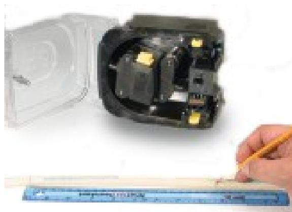
5. Open the lower spring-loaded tube clamp and locate tubing, with the first 225mm length mark aligned to the inside face of the spring-loaded part of the tube clamp. Release the clamp.
