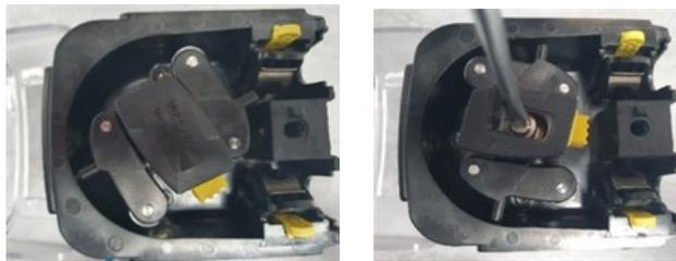
4. Remove the 4 securing fasteners.
