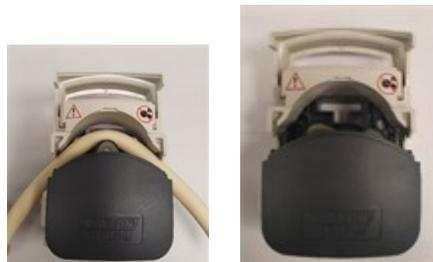
6. Lower flip top cover to fully closed position, this will automatically tension the tube correctly.
