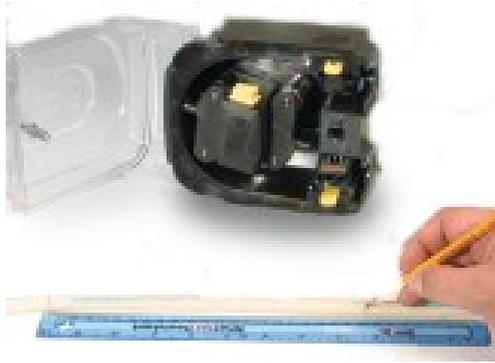
14. Open the lower spring-loaded tube clamp and locate tubing, with the first 225 mm length mark aligned to the inside face of the spring-loaded part of the tube clamp. Release the clamp.
