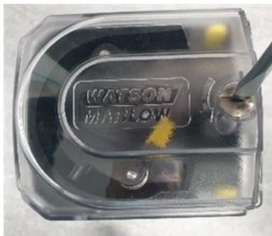
5. Open the cover to its full extent to create maximum clearance for the tube ports.
