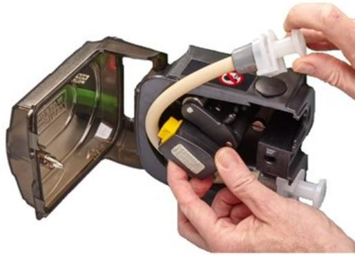
7. Place the opposite connector end of the element into the top housing. Making sure the element is not twisted and sits centrally between the rollers.
