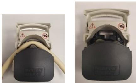
8. Lower flip top cover to fully closed position, this will automatically tension the tube correctly. Check that tubing is in the position shown. Do not add extra tension to the tube.
