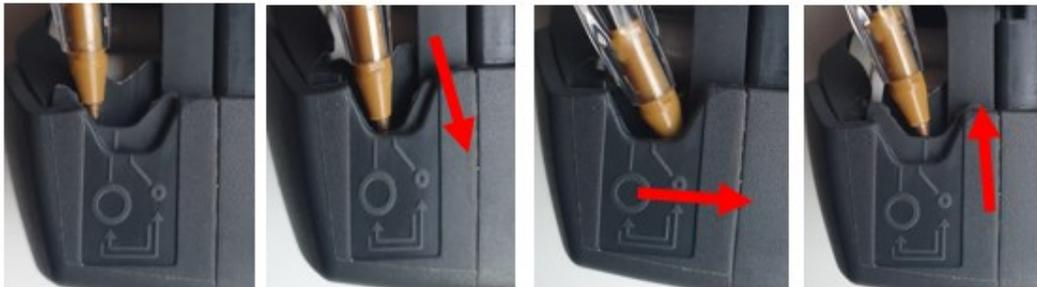
5. Press down and slightly away from the front of the pumphead, as shown above.
