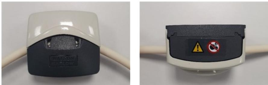
10. If using Marprene or Bioprene, retention the tubing after the first 30 minutes of operation, as the tube may grow in length during this bedding in time. Repeat all previous steps in this procedure to re-tension the tube.
