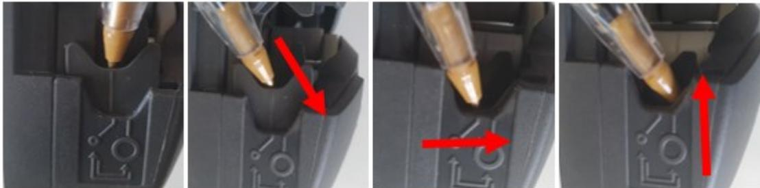
5. Press down and slightly away from the back of the pumphead as shown above.
