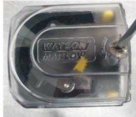
3. Remove rotor hub by lifting dust cover and removing the securing fastener.
