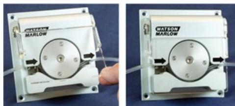
8. Connect the peristaltic tubing to the fluid path in accordance with your organisation's procedure.
