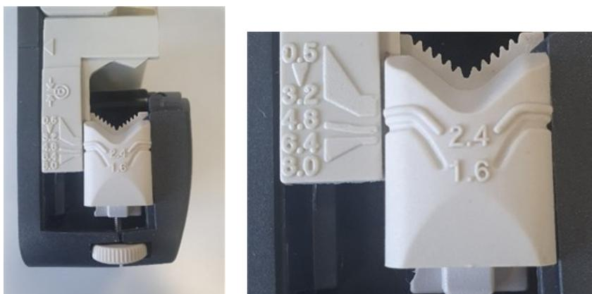
(Adjustment for 1.6 mm wall thickness and 4.8 mm tube bore size shown).
