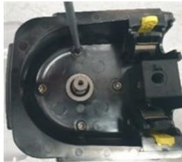
5. Remove pumphead from mounting plate and replace with new pumphead.
