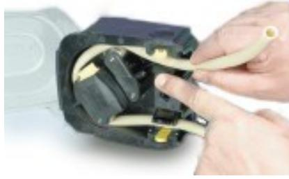
9. Check the spring-loaded tube clamps grip the tubing tightly enough to stop it moving in and out of the pumphead but must not over-squeeze the tube. Adjust the sliders to prevent tube movement during a few trial rotations of the rotor. The outer position will allow the clamps to grip the tube tightly, and the inner will grip the tube loosely
