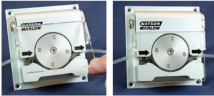
10. Connect the peristaltic tubing to the fluid path in accordance with your organisation's procedure.
