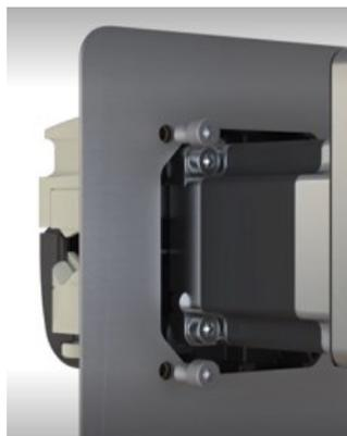
5. Torque the 4 mounting bolts using an alternating pattern to 4.6 Nm.
