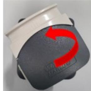
3. Place new pumphead on to mounting plate and rotate clockwise until the clip moves up and engages the pumphead.
