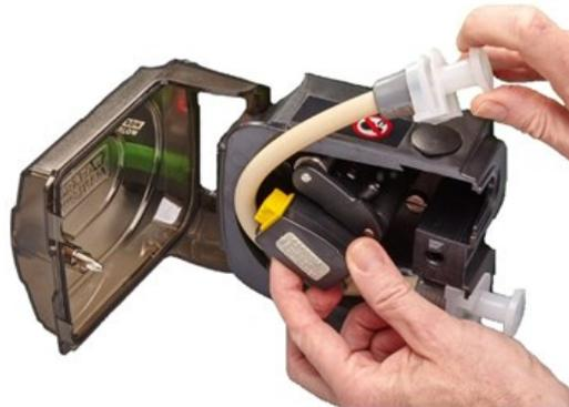
9. Place the opposite connector end of the element into the top housing. Making sure the element is not twisted and sits centrally between the rollers.
