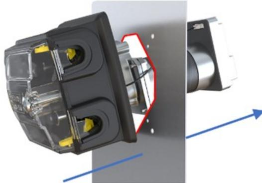
2. Pass the controller end of the pump through the aperture in the panel, until the pumphead engages the pre-drilled alignment pin holes.
