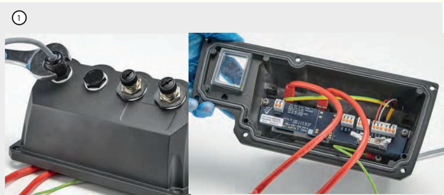
Figure 10 - Earth screening of control cables on EtherNet/IP™ NEMA module
