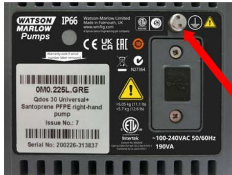
Do not use the earth bond for any other connection. Do not attempt to disassemble the Earth Bond test point
