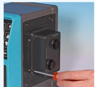
22. Use 21 mm spanner to tighten gland cap to 2.5 Nm to ensure ingress rating.
