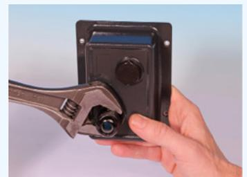
9. Loosen, but do not remove the gland cap.
