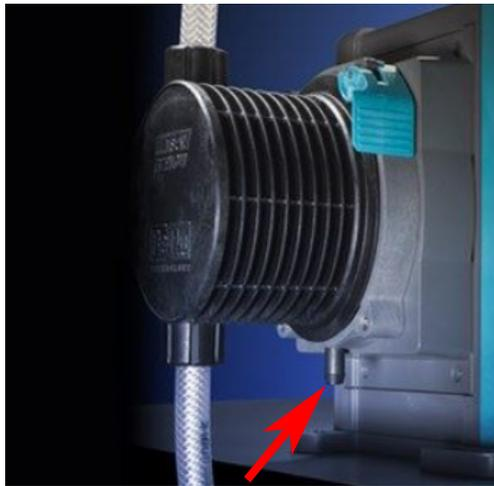
In the unlikely event of a leak detection sensor failure, the safety overflow provides a safe leak path for mixture of fluid and lubricant.
