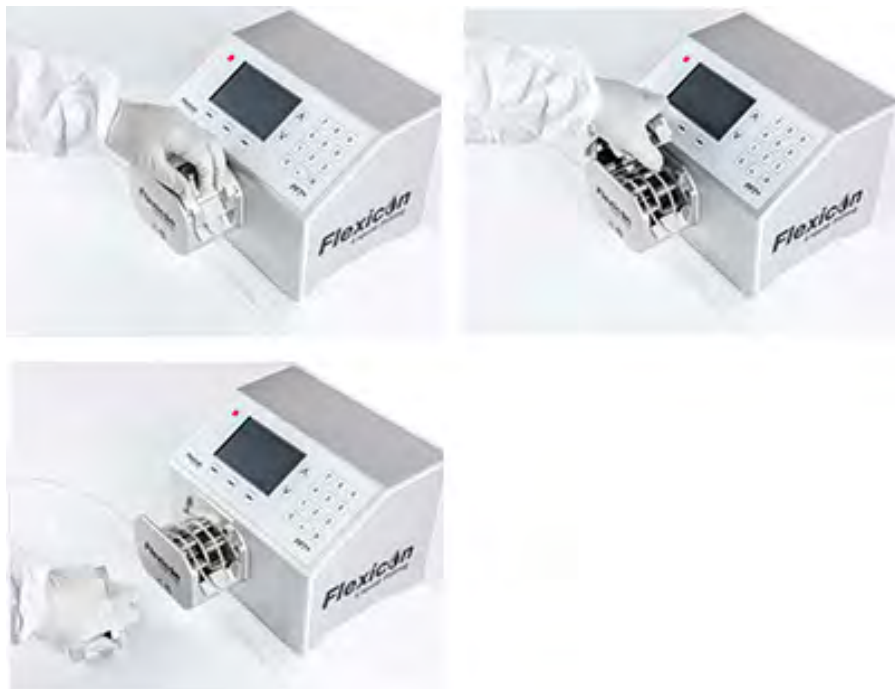
Figure 7 - Opening the pumphead
