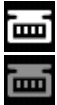
Figure 18 - Successful connection of a Mettler-Toledo ML-T balance indicated by a white icon on the Screen info bar. Successful connection of an unverified compatible balance indicated by a grey icon on the Screen info bar.
