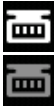
Figure 27 - Successful connection of a Mettler-Toledo ML-T balance indicated by a white icon on the Screen info bar. Successful connection of an unverified compatible balance indicated by a grey icon on the Screen info bar.
