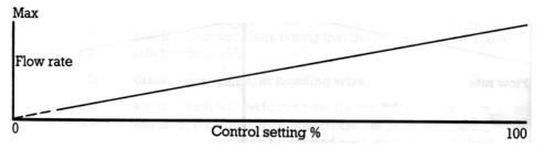
The flow rate of the 603U/R can also be controlled by any of the process control signals in common use, for instance 0-10mA as shown here.
