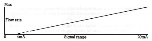
Again, the pump can be set to respond to a current signal with a signal offset and in the next illustration the signal ranges from 4mA, where flow is to be at its highest, to 20mA where flow is at its lowest.
