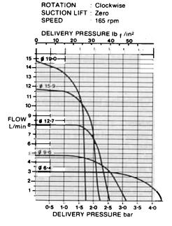
603U/Rflow rates (litre/min) against suction lift at 165rpm with clockwise rotation and zero delivery pressure
