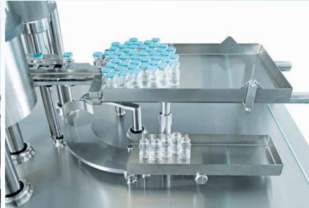
When supplied with in-line check weighing, the FPC60 offers unique dynamic prime, no intervention initial calibration and dynamic recalibration, meaning no waste in the batch start up process and confirmation every vial, from first to last, is filled within specification.
