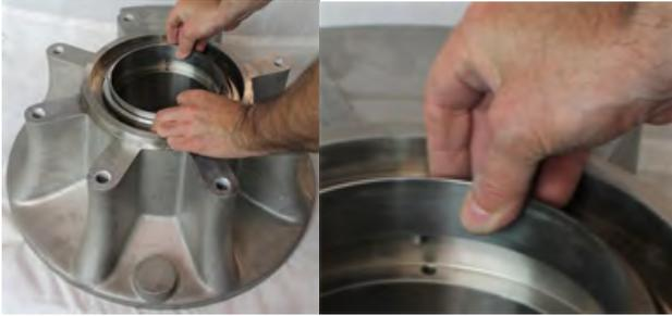
The spring assembly correctly assembled in the rear of the back housing.
