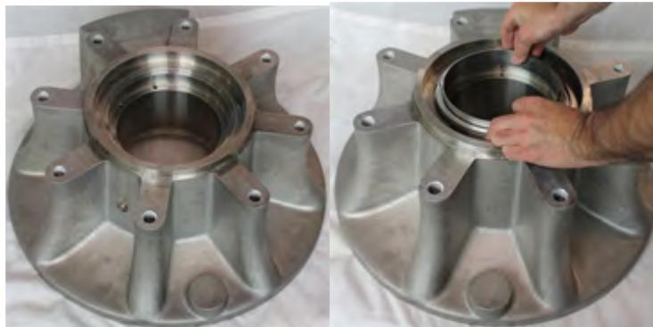
The flush ring in the back of the flange. This is used with the single mechanical seal system. A lip seal is placed in the ring in the same way as a flush ring for a flush system.
