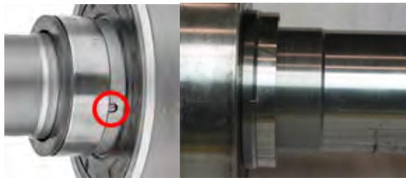
The pin correctly fitted into the notch.
