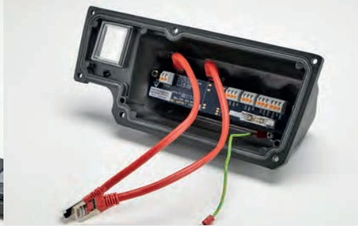
Figure 10 - Earth screening of control cables onPROFINET® NEMA module
