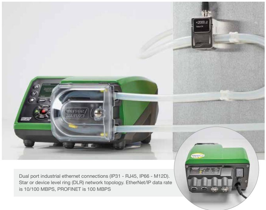
Dual port industrial ethernet connections (IP31 - RJ45, IP66 - M12D). Star or device level ring (DLR) network topology. EtherNet/IP data rate is 10/100 MBPS, PROFINET is 100 MBPS
