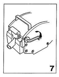
Start the pump, allow any excess tubing to work through the pumphead, and Retensioning the press the delivery end clamp down firmly. Check the tube for movement when the pump is running.
