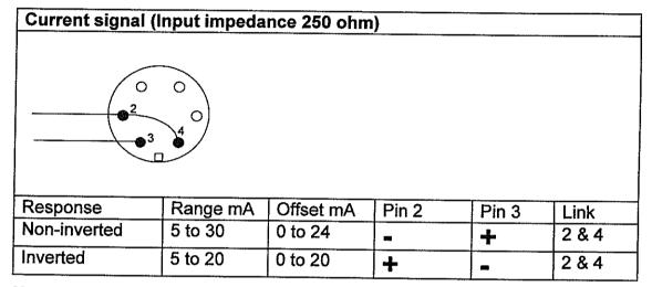
**Note:** All the connections in this section are shown viewed from the back of the plug.
