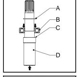
6. Place the hub (B), with the bearing side upward, on a flat surface with a hole.
