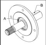
4. Push shaft (A) out of hub (B). Use a suitable pulling device.
