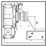
2. To correct the height loosen the 12 sets of fasteners (A).
