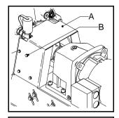
Loosen the fasteners (A) to demount the pumphead from the support set.
