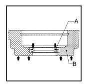
Clean the contact surfaces (A) for bearing and seal on the shaft (B). Put some grease on these surfaces.
