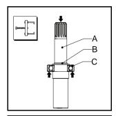
7. Remove seal (A) from hub (B). If the seal is to be replaced pliers can be used.
