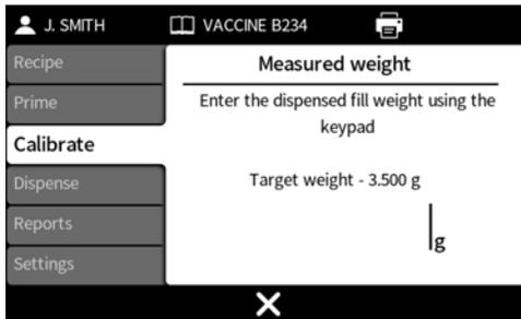
If not using a balance connected to the pump, enter the dispensed value using the numeric keypad and press
