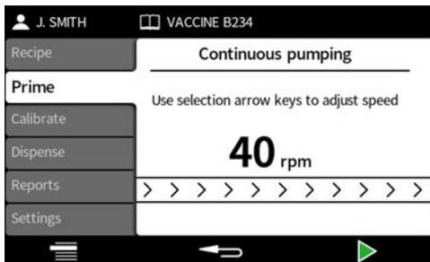
Adjust the pump speed using the up and down keys (↕/↕).
