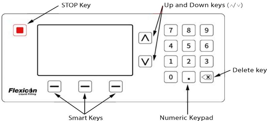
The **STOP key** will immediately stop the pump, regardless of what screen is currently displayed. If the pump is stopped part way through a fill, a message stating this will be displayed.
