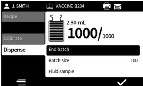
If **End batch** is highlighted press
