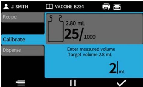
If not using a balance connected to the pump, enter the calibration value using the numeric keypad and press
