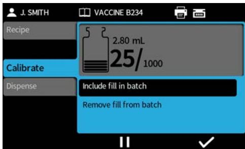
If the bottle used for calibration should be included in the batch, highlight **Include in batch** and press
