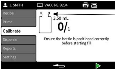
Calibration icon: The number within the vial shows how many calibration fills have been carried out since the last batch or recipe parameters change
