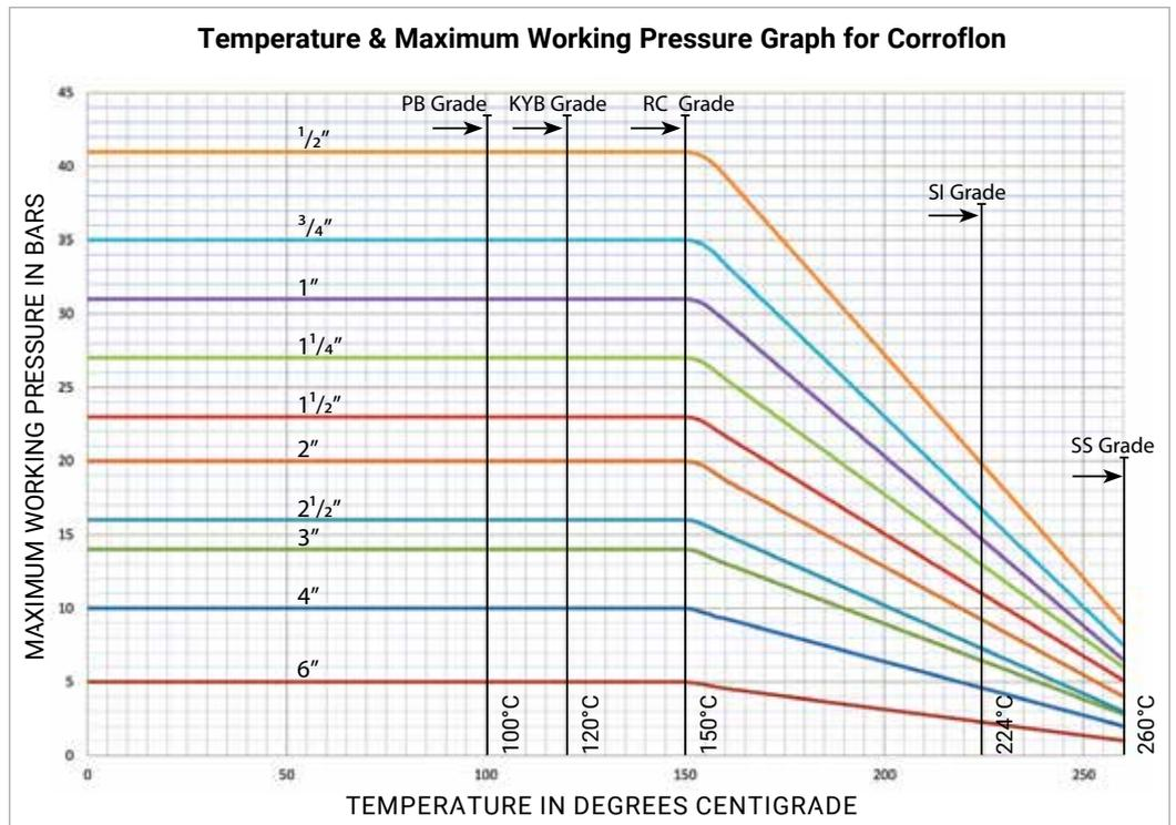
(Subtract 20°C from the above maximum temperature limits if the temperature is external to the hose).
