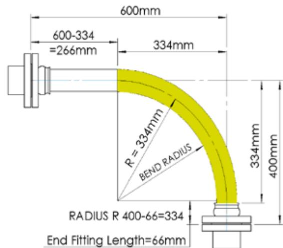
Note: The bend radius is measured to the inside edge of the hose, For the minimum bend radius refer to page 6.
