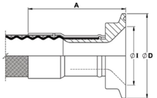
\*Fitting Lengths listed are for Corroflon braided only hose grades (SS, PB, HB, KYB). Approximately 33% longer lengths apply to the rubber covered hose grades (RC, SI).
