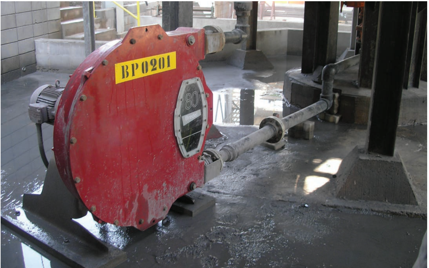
Above: Breidel 80 hose pump in thickener underflow application
