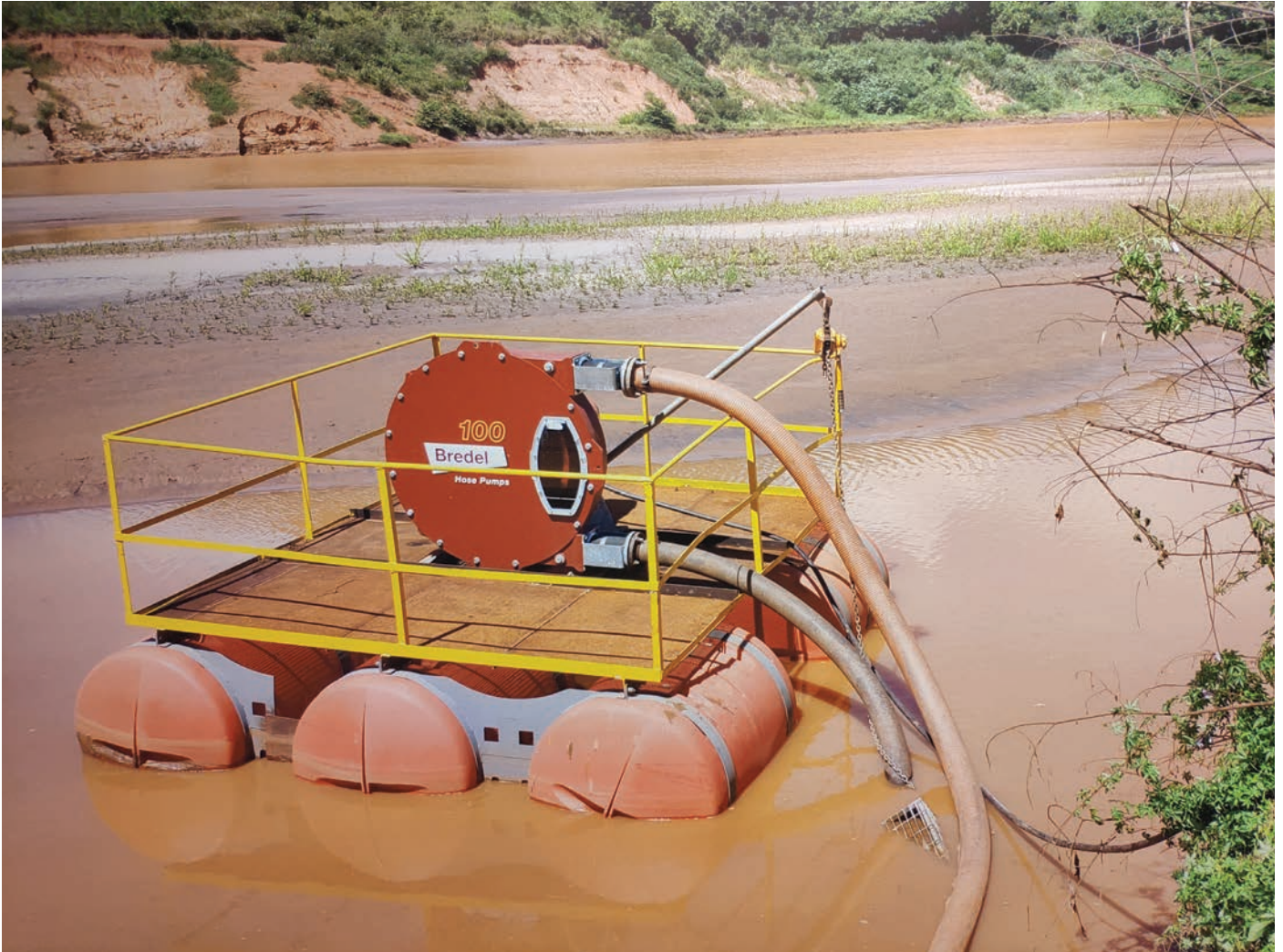
Above: Grit and solids laden water being pumped for mining operations
