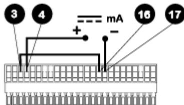
For current modes the same DC source can be used in conjunction with a DC milliampere meter, (maximum 32mA). (See 25 pin terminal strip detail.) Circuit impedance 250Ohms. Polarity set for non-inverted response. Reverse polarity for inverted response.
