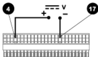
be used in conjunction with a DC voltmeter, (max 30V DC). (Refer to the 25 pin terminal strip wiring detail as an example of control circuitry.) Circuit impedance 100kOhms. Polarity set for non-inverted response. Reverse polarity for inverted response.
