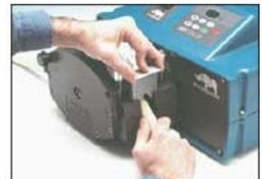
When using Marprene continuous tubing, after the first 30 minutes of running, re-tension the tube in the pumphead by releasing the tube clamp on the delivery side a little and pulling the tube tight. This is necessary to counteract the normal stretching that occurs with Marprene which can go unnoticed and result in poor
