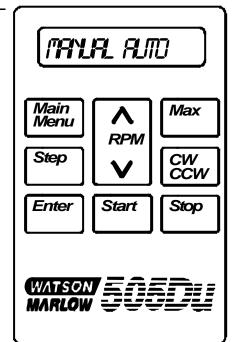
The 505Du can be operated under manual control, analogue or digital RS232 auto-control, with remote or TTL control of direction and stop/start.
