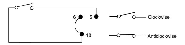
A remote potentiometer with a nominal value of between 1k and 5k with a Speed minimum of 0.25W should be wired as shown. When using a remote potentiometer, do not apply a voltage/current control input signal at the same time. The drive must be calibrated for 0-12V control as described in the auto analogue section. Alternatively, the potentiometer may be used for the calibration procedure, instead of using the minimum and maximum signals, if it is set to its minimum and maximum positions.
