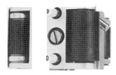
Should it appear that the roller arms are not equally adjusted and it is desired that the original factory setting be restored, turn the adjusting screws until both rollers are just touching the track, then tighten each by 3 1/2 turns, thus restoring the gap to the original 2.8mm setting.
