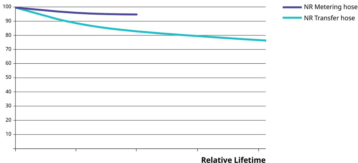
Typical performance test conditions: pumping water at 18°C (64°F) at 5 bar (73 psi) and 50rpm
