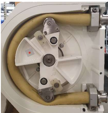
Rocker assemblies shown locked for bi-directional pumping
