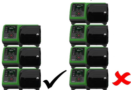
Figure 2 - Stabling af pumper
