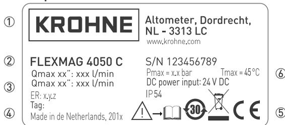
Figure 2-3: Example of nameplate
