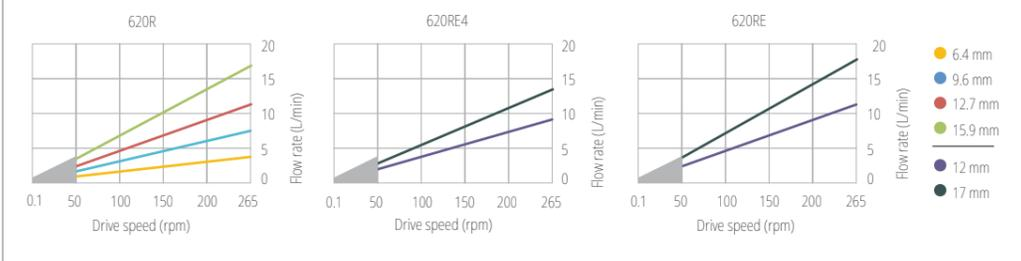
• Limited to 2 bar below 50 rpm. Flow rate varies with tube material, discharge pressure, suction and viscosity
