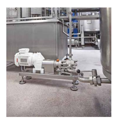
Certa by MasoSine outperforms lobe pumps in critical processing applications. The sinusoidal rotor design delivers a lower shear, gentle pumping action that safely transfers delicate products without risk of degradation.
